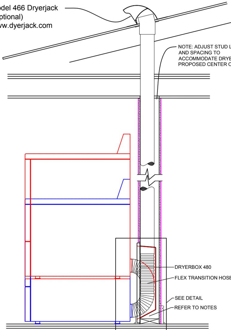
NOTE: ADJUST STUD LOCATION AND SPACING TO ACCOMMODATE DRYERBOX AT PROPOSED CENTER OF DRYER.
