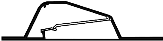
RCDV - Roof Cap side view (cutaway)
